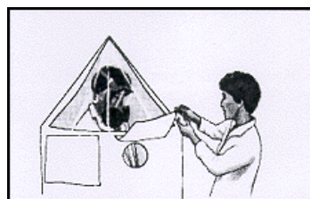
Qualitative Fit Test Chamber
